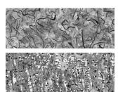
The microstructure will contain Type VII, A, size 4-6 graphite as defined in ASTM A247. The matrix is fully pearlitic. The edge or rim will consist of Type D, size 4-6 graphite in a matrix that is a combination of pearlite and ferrite. Chill carbides will be less than 5% in any field at 100x and are well dispersed.
