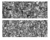
The microstructure will contain Type VII, A, size 4-6 graphite as defined in ASTM A247. The matrix is fully pearlitic. The edge or rim will consist of Type D, size 4-6 graphite in a matrix that is 80% pearlite. Chill carbides will be less than 5% in any field at 100x and are well dispersed.
