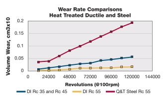
Data is based on 3 pad specimens on 52100 hardened steel disks, dry conditions, 150 lbs force
