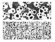
The microstructure consists of Types I & II nodular graphite as defined in ASTM A247. The matrix is ferrite with approximately 5-25% pearlite. The edge or rim will have a higher nodular count and will be mostly ferrite. Chill carbides will be less than 5% in any field at 100x and will be well dispersed.
